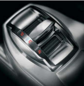
Alfa Romeo D.N.A. (vehicle's dynamic control switch)
