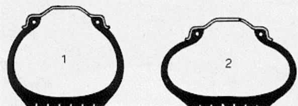
Fig. 13 - 1. Correct inflation - 2. Insufficient inflation
