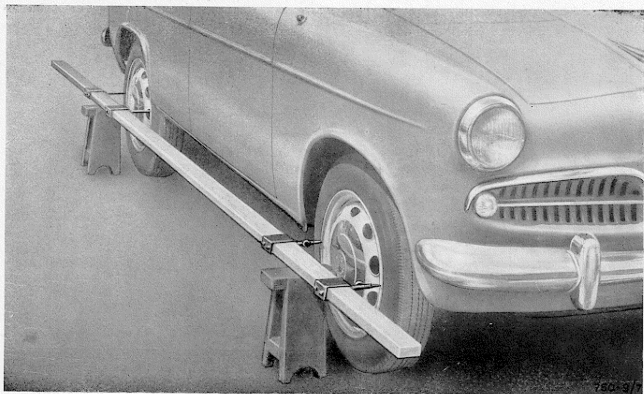
Fig. 7 - Measuring front-wheel toe-in with the wheel rims taken as reference points
