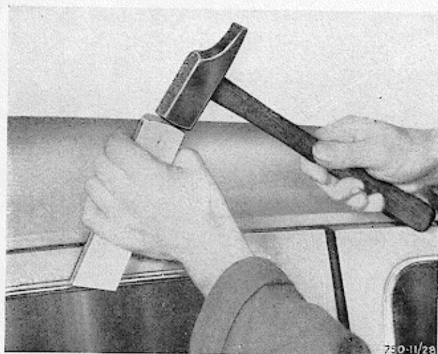
Fig. 27 - Removing the metal frame from a side window
