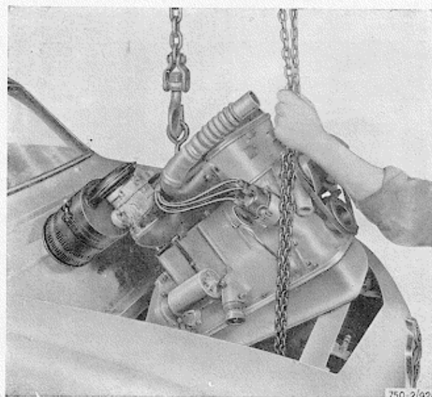
Fig. 92 - Taking off the engine-gearbox unit (transmission) from the car
