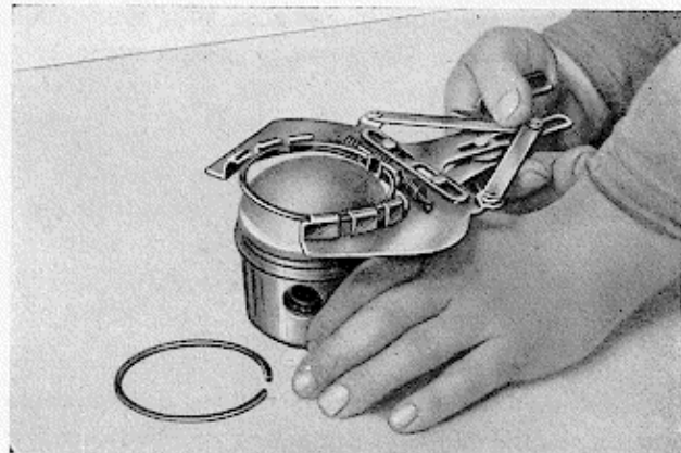
Fig. 68 - Dismantling the piston rings
