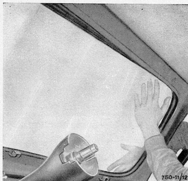
Fig. 11 - Removing the windshield glass
