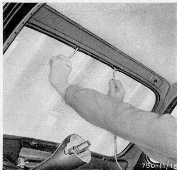
Fig. 17 - Simultaneously removing the cord and fitting the rubber surround over the edge of the opening in the car body
