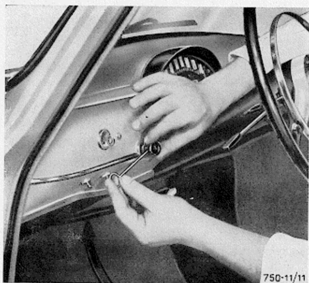
Fig. 10 - Removing the driving-light switch knob
