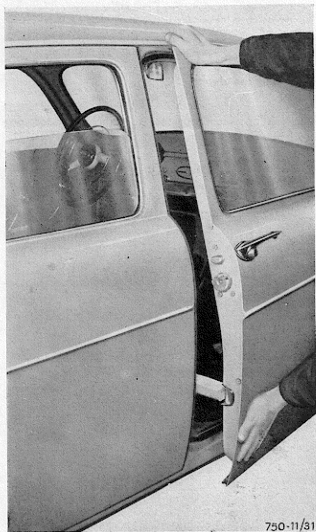
Fig. 30 - Correcting a badly-fitting door to ensure that the rubber seal adequately excludes water and dust
