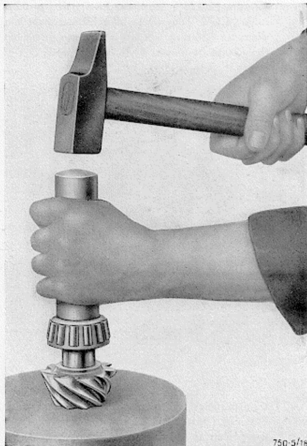
Fig. 18 - Mounting the inner race of the rear bearing on the bevel pinion, using tool 6121.07.220
