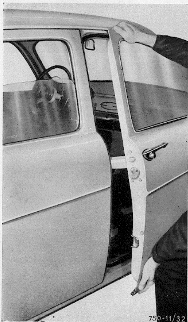
Fig. 31 - Correcting a warped door to ensure a close fit
