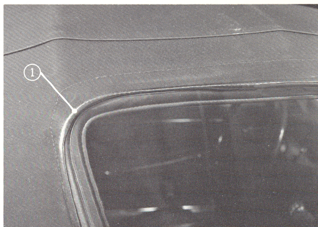
Window too high, pinching top piping.
